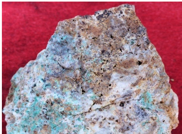
Epithermal quartz breccia assayed 2.60% Cu, 6.0g/t Au
