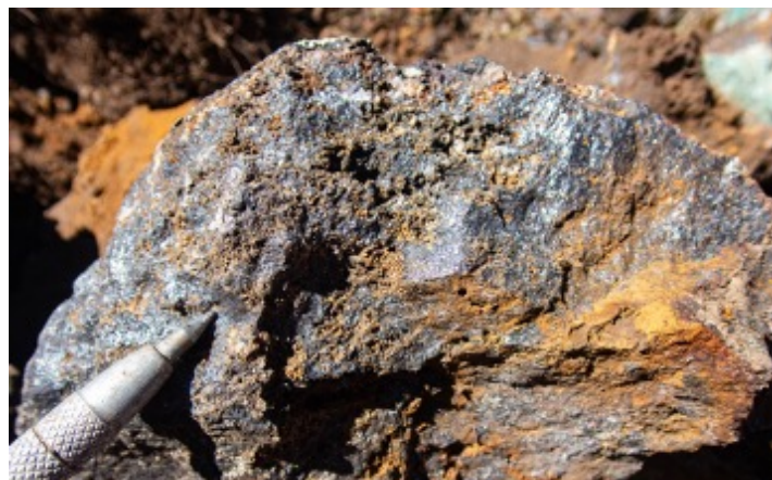
Magnetite skarn, assayed 1.13% copper and 0.17g/t gold
