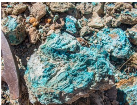
Garnet skarn with copper oxides, assayed 2.82% copper
