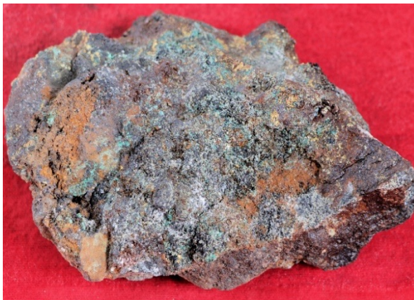
Skarn with bornite assayed 2.61% Cu, 0.11g/t Au
