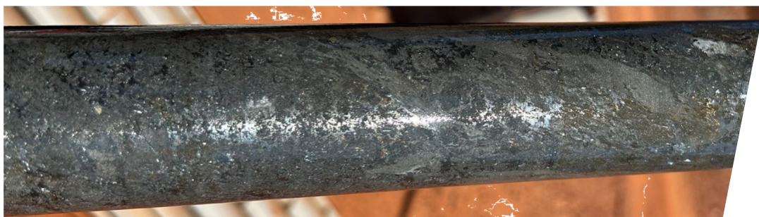
Core from drillhole EHDD25001 (~240m depth) showing semi-massive sulphide mineralisation (pyrite-pyrrhotite-boulangerite ( Pb_5Sb_4S_{11} )) 1
