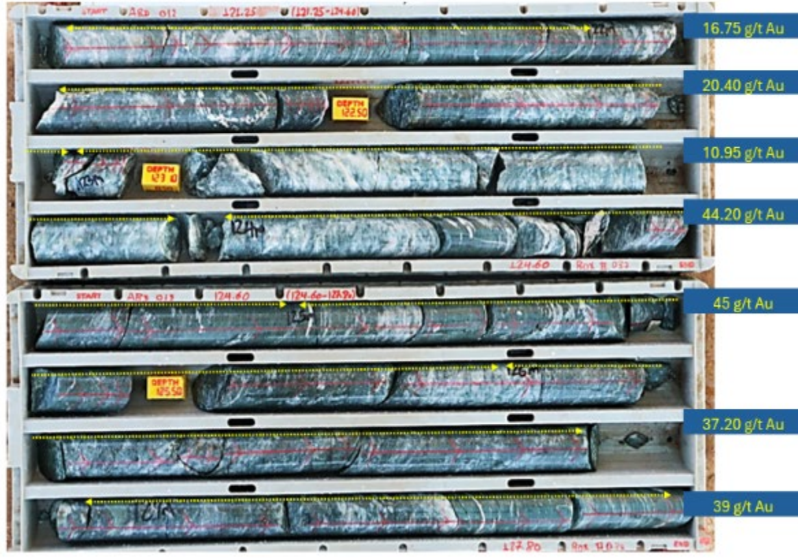
Core Photographs, Drillhole: ABD012: 121.25-127.80m
