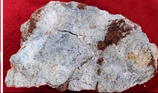
Phyllic altered diorite porphyry assayed 1.41% Cu and 0.98g/t Au
