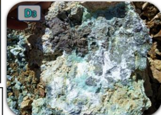
RC21902, select sample of Pyrite – enargite + copper oxides from structure in D1 Au: 0.97 g/t, Ag: 14.7 g/t, Cu: 0.36%, Mo: 5.9ppm
