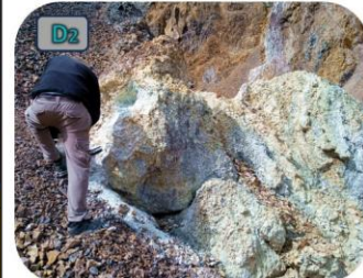
RC21903, channel sampling of 6m-wide structure with adv. Argillic alteration. Pyrite, enargite, copper oxides 1m channel sample at 0.53 g/t Au, 17.5 g/t Ag, 861ppm Cu, 6.8ppm Mo
