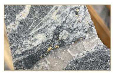
Native 'free gold' in drill core from hole GS2335 (3.1-metres at 39.5 g/t Au from 142.3m)
