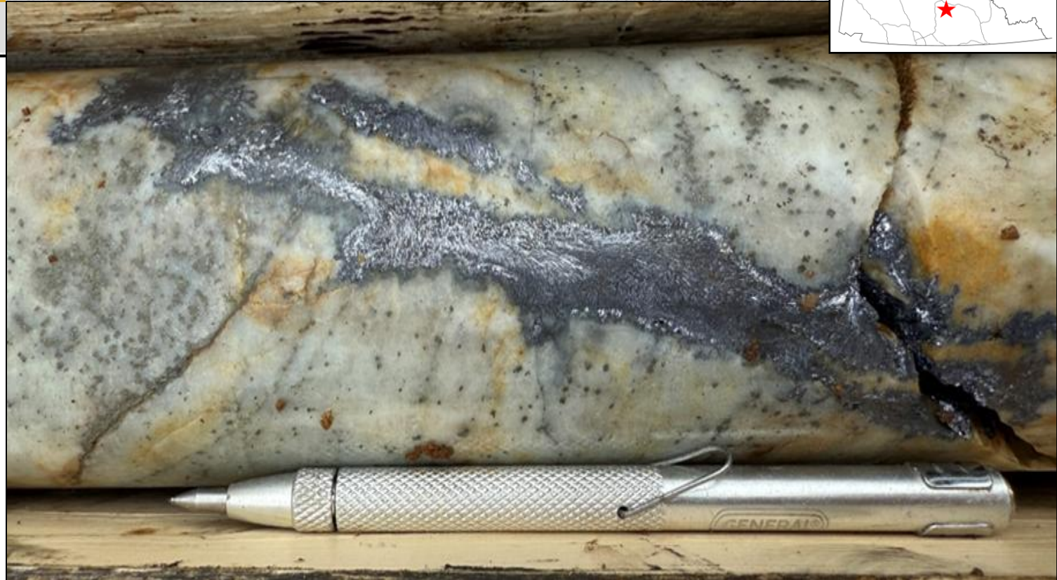
FIGURE 2- HOLE SR25-003 AT 18M SHOWING GALENA VEIN CUTTING QUARTZITE WITH DISSEMINATED PYRITE-ARSENOPYRITE.
