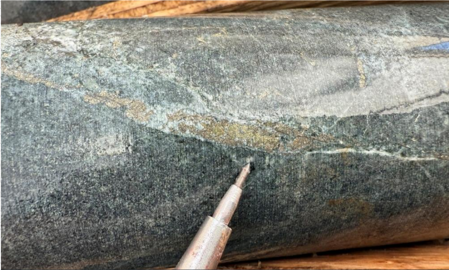
DIORITE WITH QUARTZ-PYRITE-CHALCOPYRITE VEINING AT 51.7M IN HOLE AZ25-004.
