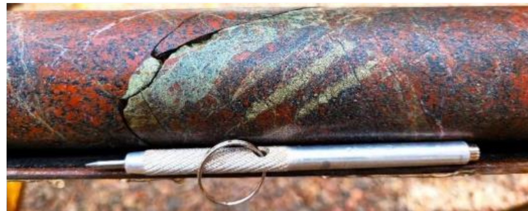
Altered and brecciated "green rock" (epidotization and chloritization) with pyrite veinlets: DDSTH-0001.
