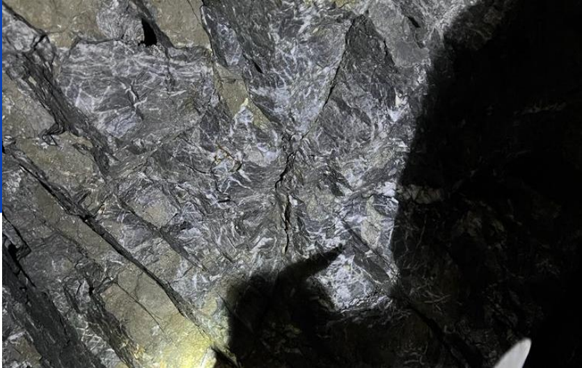
"Sheeted" sulphide ore. Fault breccia hosted in carbonaceous schist
