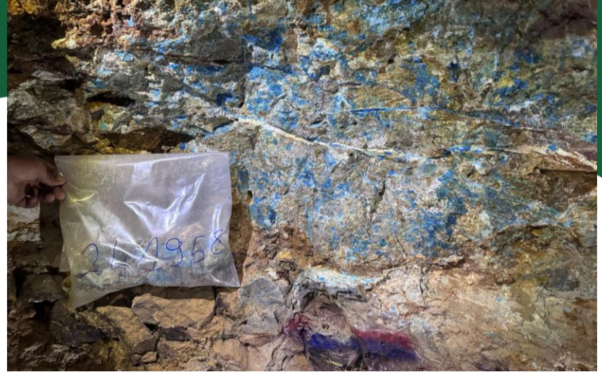
Cleavage-parallel azurite in "wall-rock" adjacent to vein-breccia mineralization from the Eastern Breccia Zone
