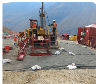
Minimizing our environmental footprint and protecting+preserving land+water by using membranes to protect against drill-site spills and to recover-recycle used water as well as protecting indigenous plant species.
