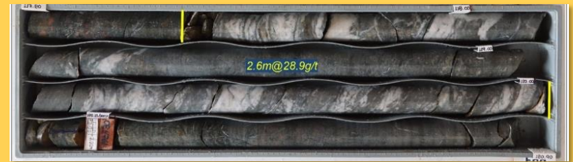
High-grade zone in DDH271 which returned 2.6m @ 28.9 g/t gold including 1m @ 64.6 g/t gold
