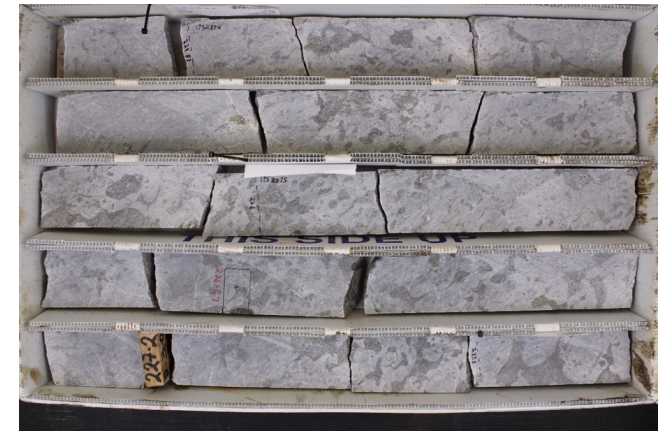
B21C-016: 227 m. Patchy pyrophyllite "gusano" alteration textures
