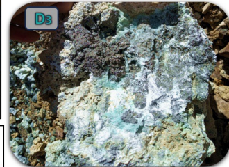
RC21902, select sample of Pyrite – energite + copper oxides from structure in D1 Au: 0.97 g/t, Ag: 14.7 g/t, Cu: 0.36%, Mo: 5.9ppm
