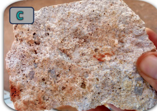
RC21886, Residual quartz-vuggy silica with adv. argillic alteration, silica – alunite. 1.5m at 0.86 g/t Au, 22.1 g/t Ag, 51.7 ppm Cu, 17.2 ppm Mo, 115 ppm Sb
