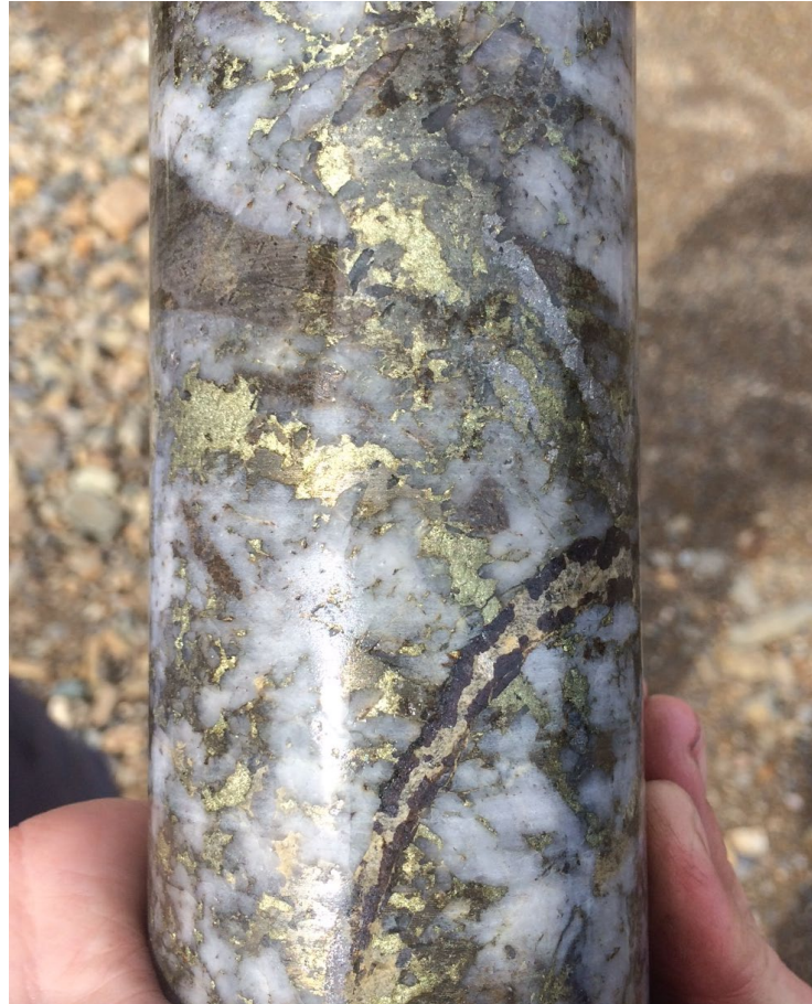
Chalcopyrite, wolframite and pyrrhotite in drill core
