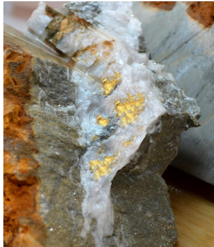
Photo of coarse visible gold in a quartz vein channel sample, Trench 3 – Croteau Bouchard Shear Zone, Croteau property. Grab sample assay, 92.57 g/t gold: channel sample average assay, 14.37 g/t Au/7.5 m.
