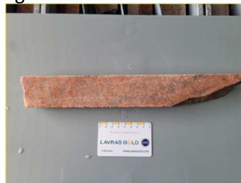
Moderate to strongly altered granodiorite: Salmon pink metasomatic alteration front altering original granodiorite.
