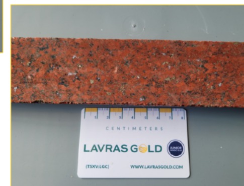
Episyenite with millimetre scale cross-cutting pyrite veinlets, 1 metre interval grading 1.6 g/t gold
