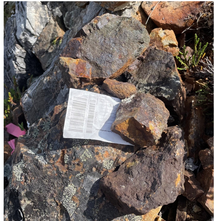
Rock Sample K654501 of mineralized skarn horizon grading 14.1 g/t Au and 4,260 ppm Cu.
