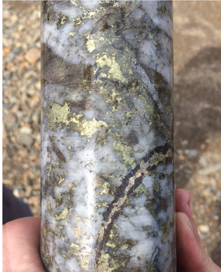
Chalcopyrite, wolframite and pyrrhotite in drill core
