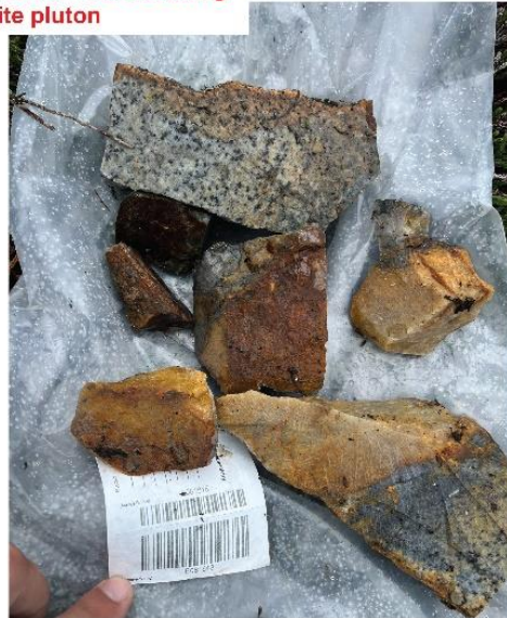
Sphalerite (2%), pyrite (1%), molybdenite and bismuth in 15 cm quartz vein crosscutting granodiorite pluton
