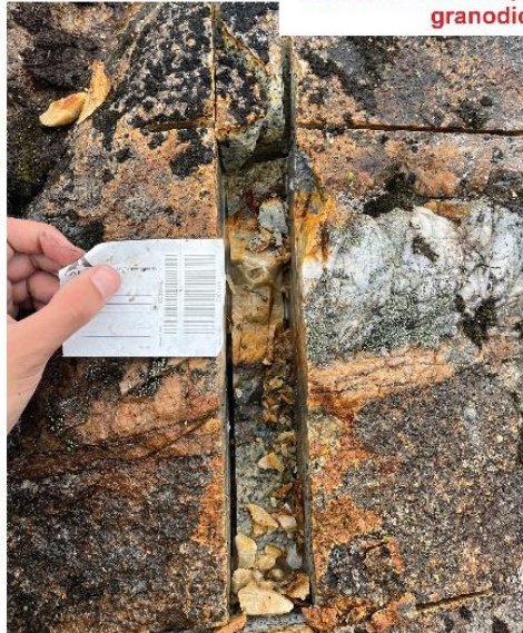
Sphalerite (2%), pyrite (1%), molybdenite and bismuth in 15 cm quartz vein crosscutting granodiorite pluton
