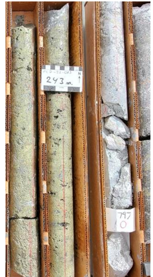
Photo of drill core from drill hole FDC-22-013 at the Copper Prince breccia.
