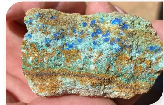
Copper oxides replacing chalcocite in outcropping sandstone (this sample has not been assayed by a certified laboratory)
