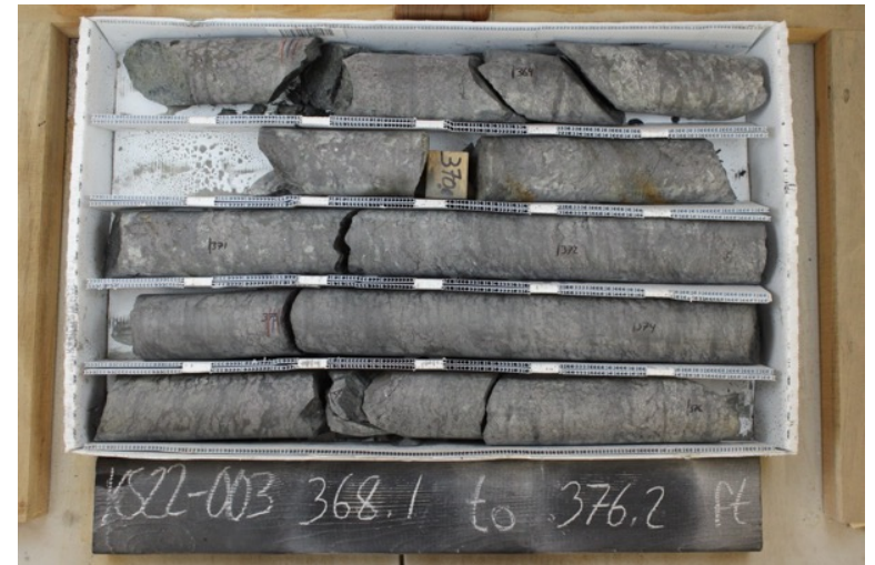
KS22-003 Core photo of magnetite rich ultramafic with nickel sulfide
