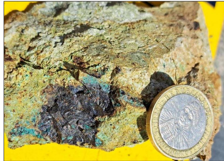
Sample # 8615 grading 5.37% Cu from the Lucero Prospect 2 .
