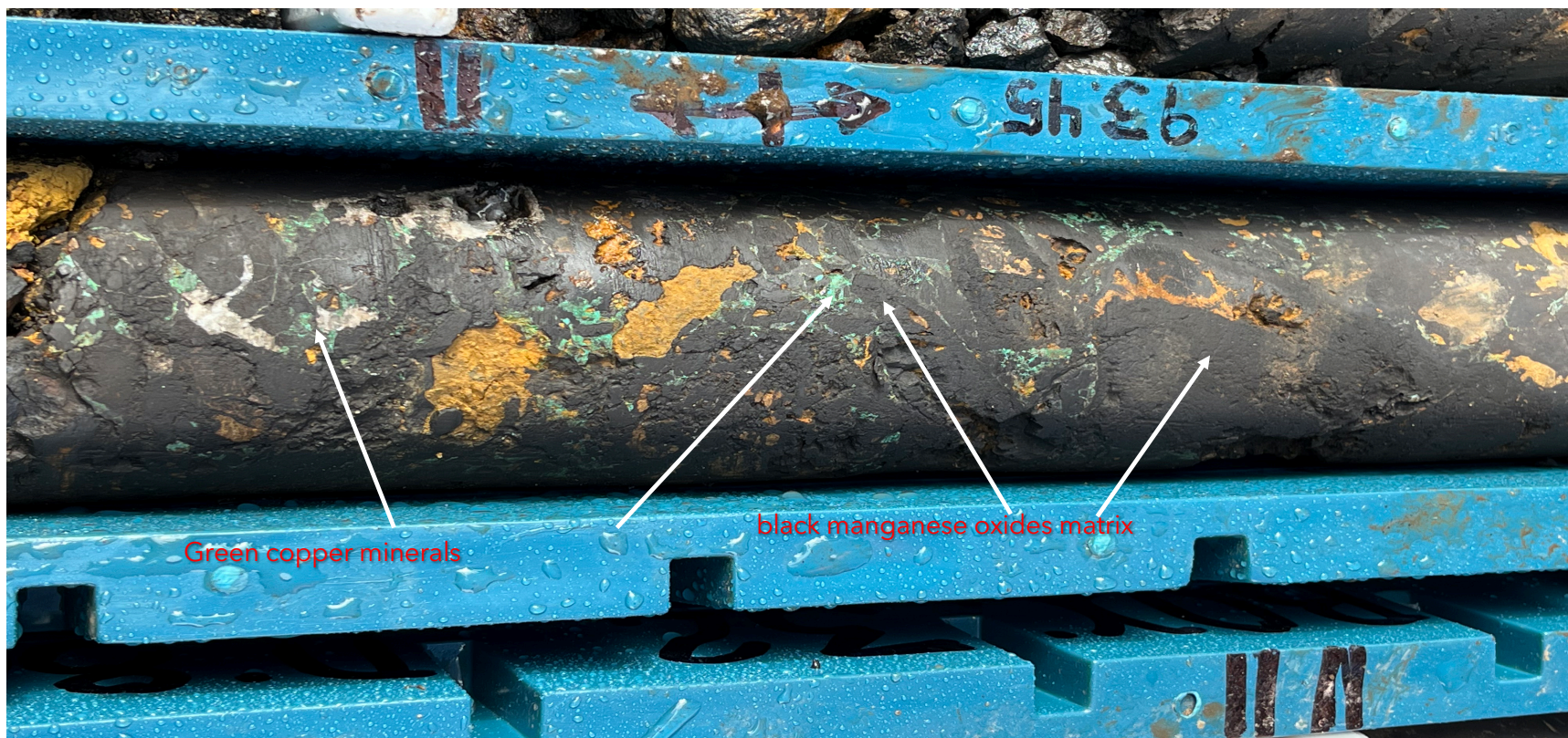
Silver and copper (green) mineralization is hosted within a manganese oxide matrix (black)
