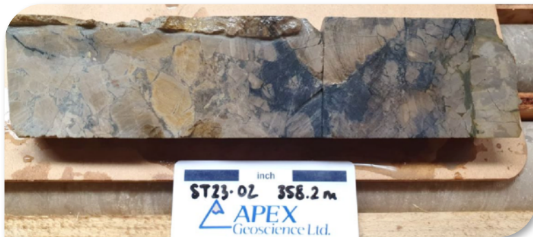
High-grade copper – Drilling confirms high-grade potential (Strong chalcocite breccia fill and veining in ST23-02).
