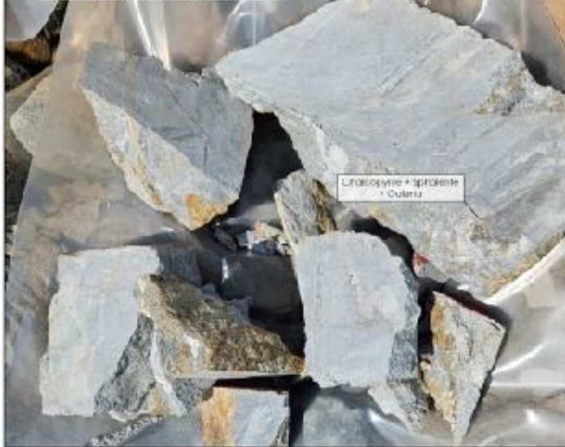
B ST1 12963: 0.73m Channel Grab Stockwork Quartz-Chalcopyrite-sphalerite-galeru
