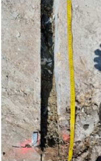
A ST1 12963: 0.73m Channel Grab Stockwork Quartz-Chalcopyrite-Sphalerite-Galeru
