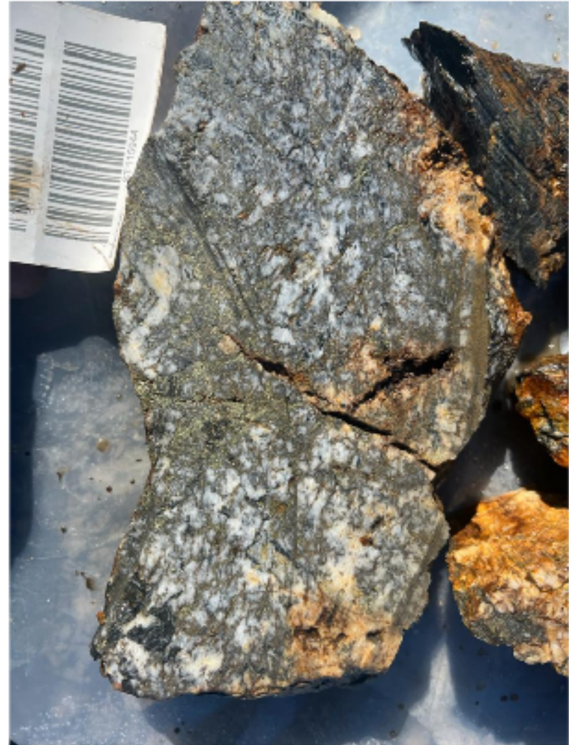
Samples from brecciated shears and veins with massive chalcopyrite and pyrite
