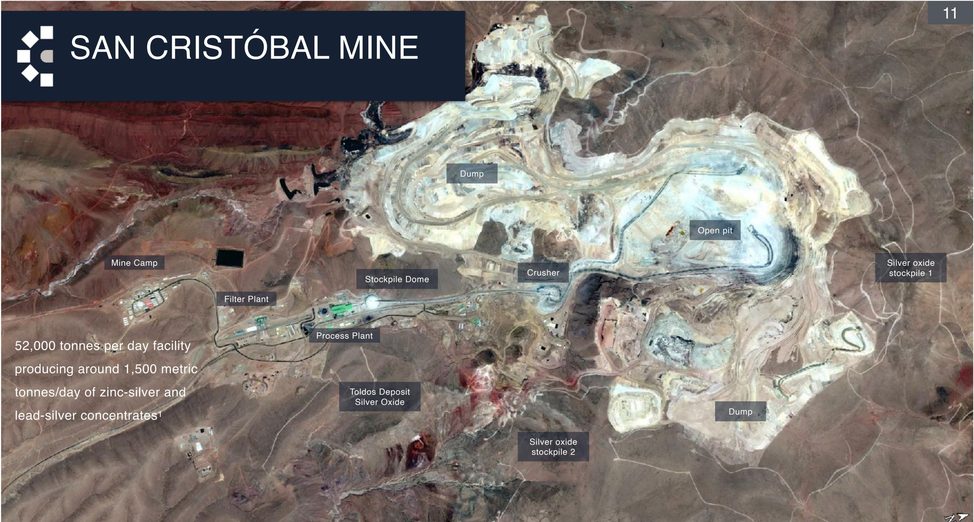
52,000 tonnes per day facility producing around 1,500 metric tonnes/day of zinc-silver and lead-silver concentrates<sup>1</sup>
