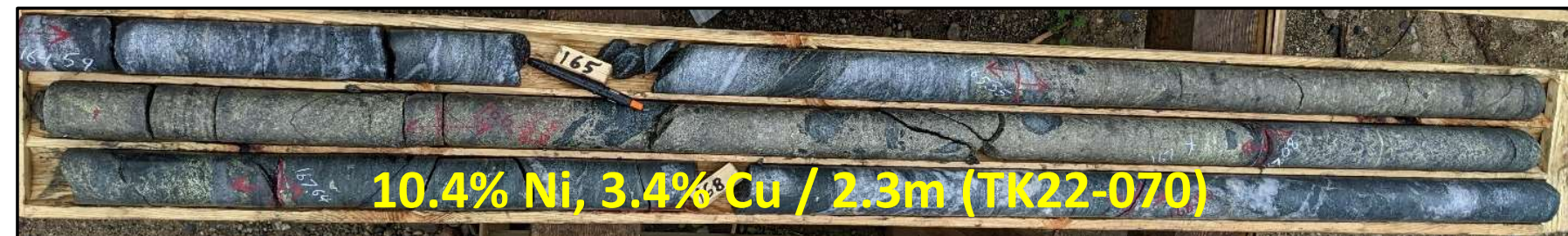
2.1m vein of massive sulphide (Pn-Cpy-Po) at WP.
