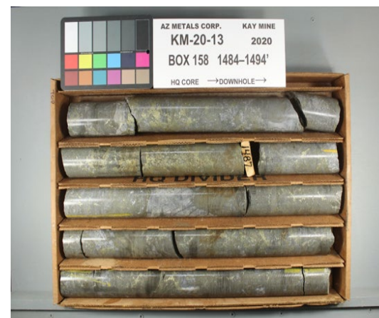
Chalcopyrite and sphalerite mineralization
