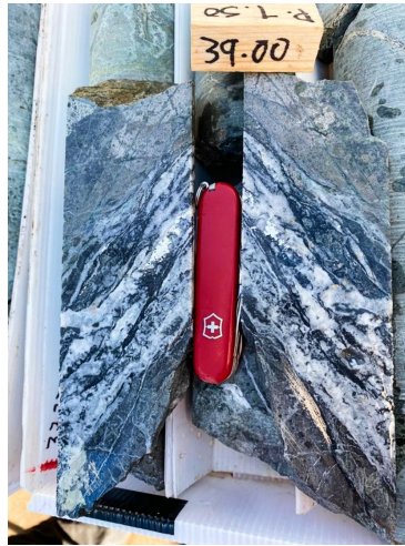
Section of BA21-30 core showing native silver mineralization
