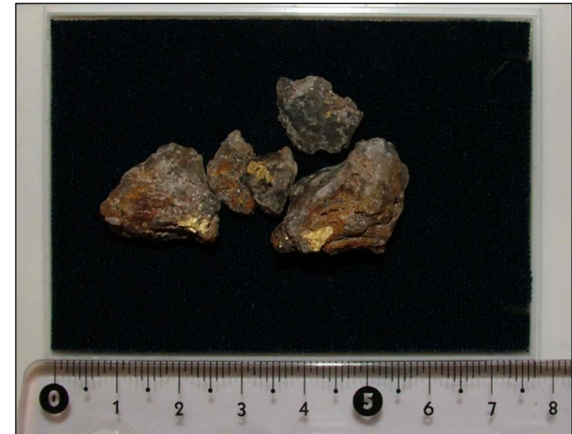
Gold in qtz pebbles panned out of the till in the main boulder train
