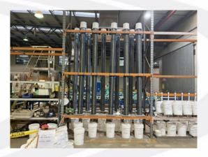
Refer Slide 22 Results obtained from column leach tests across Apollo Hill's geology, grade range and geography at P<sub>100</sub> 8mm HPGR Crush.
