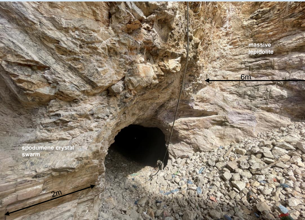
Spodumene crystals (left) grading to lepidolite (right) in Thor's Oyo State Project
