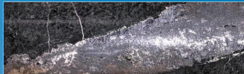
CS-19-08-W02 (70,380 gpt Ag over 0.3 m) Massive native silver in hairline silver-filled fractures in CS-19-08-W02 @ ~418 m vertical depth
