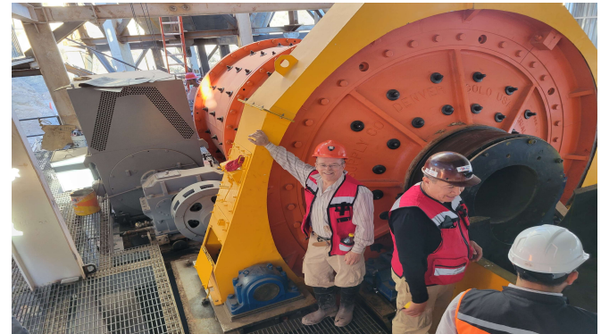
First Ball Mill has been installed
