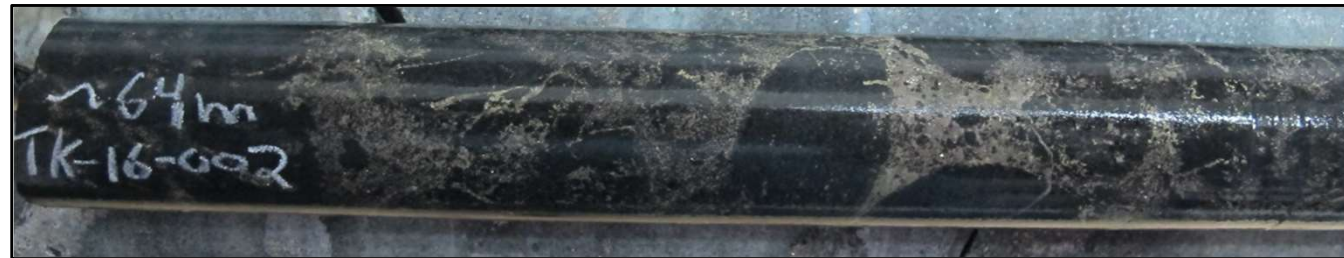
Breccia hosted, primary-type semi-massive sulphide textures in RJ Zone. High-tenor Ni sulphides (Pn)
