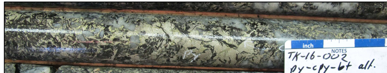
Remobilized Pn-cpy within Tonalite with at RJ Zone.
