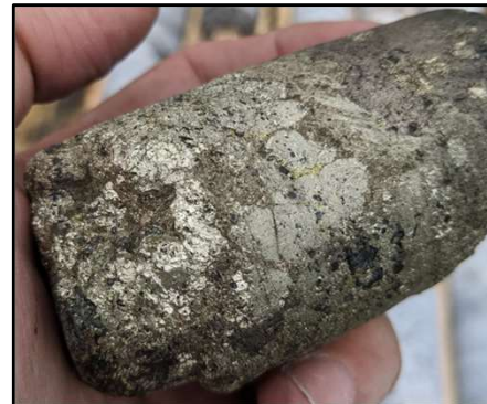
Close-up of coarse pentlandite "eyes" in massive sulphide veining at WP.
