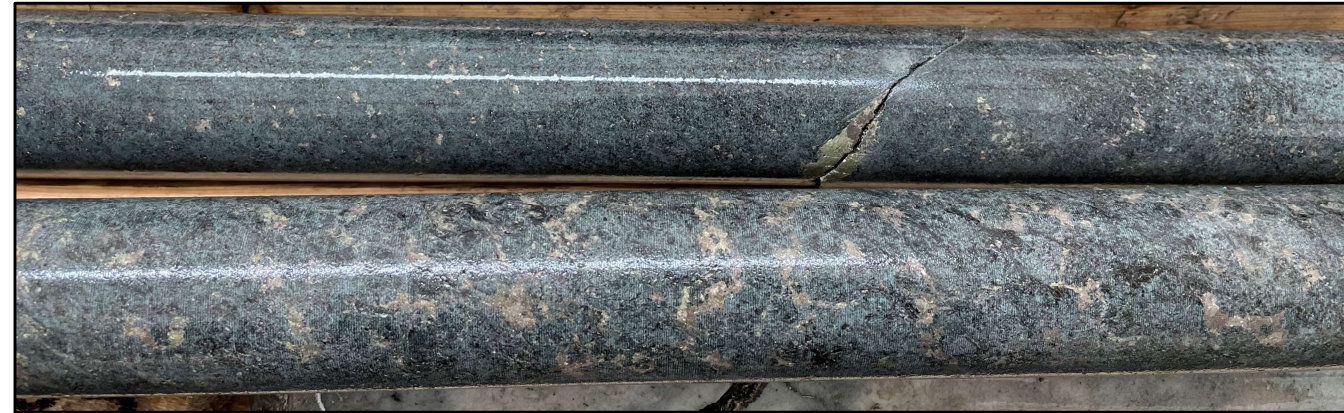
Blebby to interstitial, primary-type sulphide textures in RJ Zone. High-tenor Ni sulphides (Pn)
