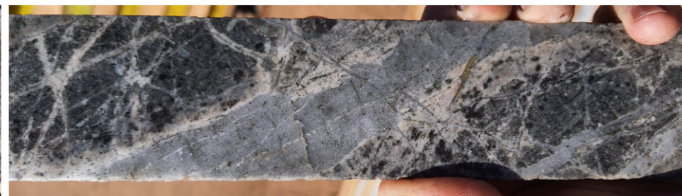
1239m: Porphyritic diorite, biotite- magnetite-potassium feldspar alteration with quartz-magnetite-chalcopyrite-pyrite in veins and disseminate chalcopyrite and pyrite
