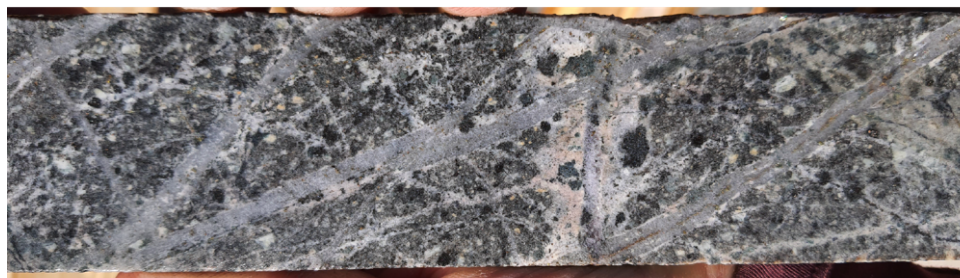
1233m: quartz-diorite, biotite-magnetite potassium feldspar alteration with quartz- magnetite-chalcopyrite-pyrite in veins and disseminate chalcopyrite and pyrite
