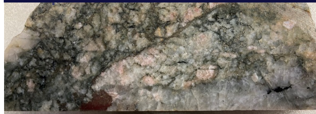
Brecciated monzonite with sericite, chlorite and quartz (5.83 g/t Au)
