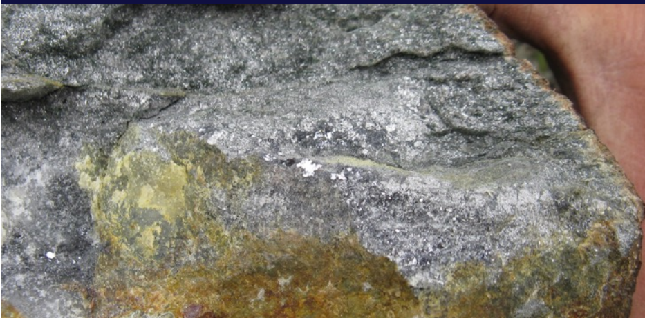
Typical arsenopyrite- and gold-rich sample from shear zones around the Menarik Complex (up to 58 g/t Au and 853 g/t Ag)
