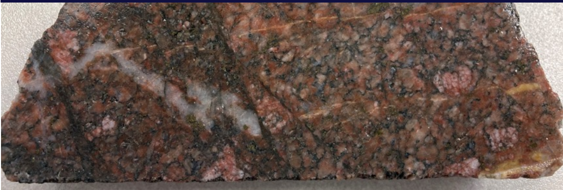
Strong alteration in hematite, chlorite, silica, sericite and carbonate in the monzonite
