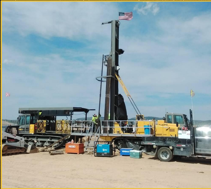
Sonic drill rig used at Oro Cruz Project in January 2021
