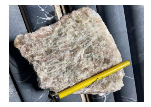
Spodumene crystals in Sample 361716 (1.82% Li<sub>2</sub>O)
