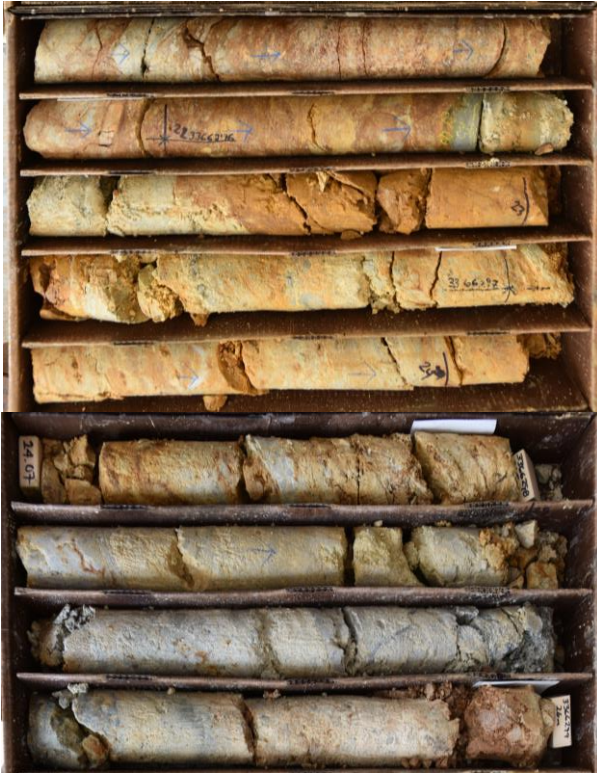
Drill Hole NA19-169 21.3-26m 4m @ 14.98 gpt Au in strongly clay altered/ oxidized fault gouge.
