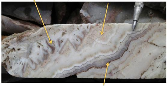
Crustiform banded quartz phases, including a chalcedonic quartz phase
