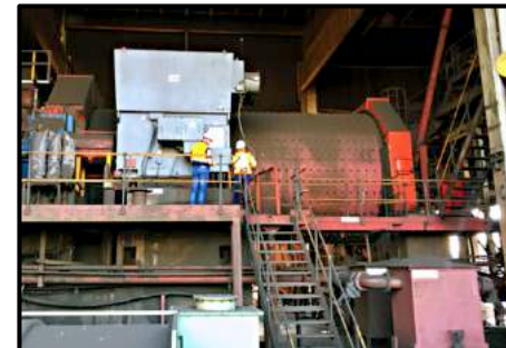
2.5MW Ball mill (photo taken at Rustenburg during independent inspection by METS).
