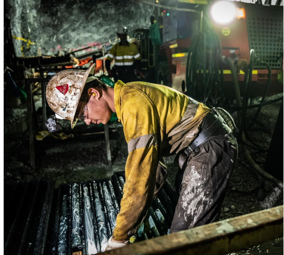
KOTH underground diamond drilling Driller's offsider cleaning core after retrieving from core tube, before placing in tray
