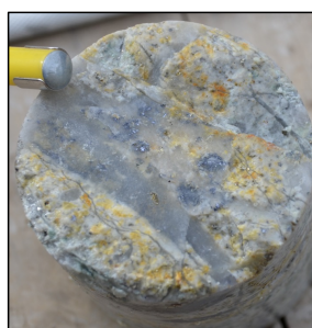
CK18-2 : altered stock work porphyry dike at 25 m with Mo, cpy & py
