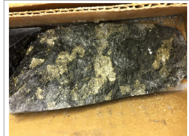
PGE-Nickel-copper mineralization in drill core from the lower Stillwater Complex at Stillwater West
