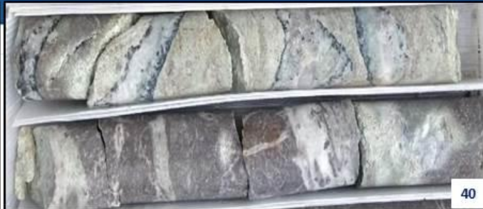
1.6m @ 8.96 gpt Au, 1,078.7 gpt Ag, or 1,750 gpt AgEq including 0.5m @ 26.6 gpt Au, 3,210 gpt Ag, or 5,205 gpt AgEq
