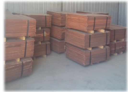
Stacks of copper cathode produced from Solvent Extraction & Electrowinning process
