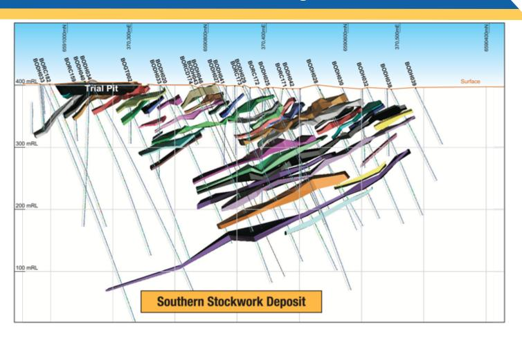
Boorara Gold Project Southern Stockwork Long Section Wireframes Mineralised Vein Arrays +1g/t Looking NE 060 +- 80m
