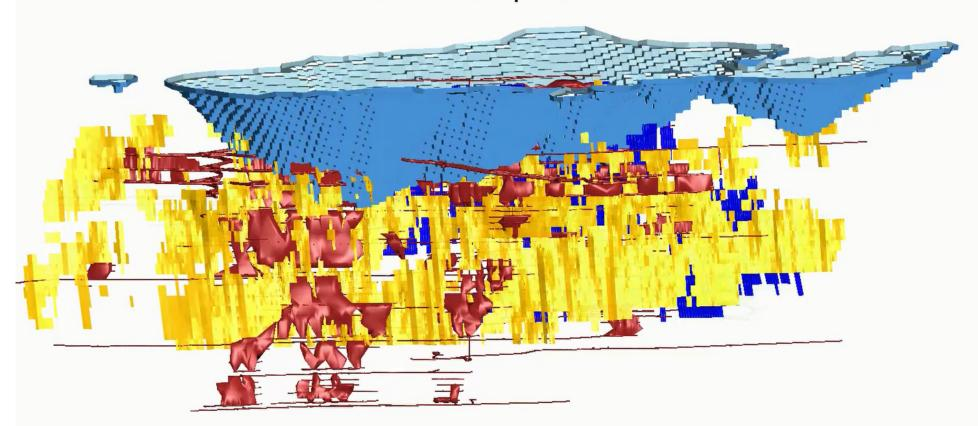
Blue: West Lode UG 3.0g/t Optimised Shapes Underground bulk mining assessments to be completed
