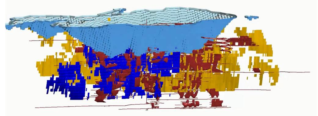
Blue: West Lode UG 3.0g/t Optimised Shapes Underground bulk mining assessments to be completed
